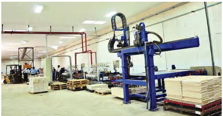
Rectification and Chamfering of tiles
