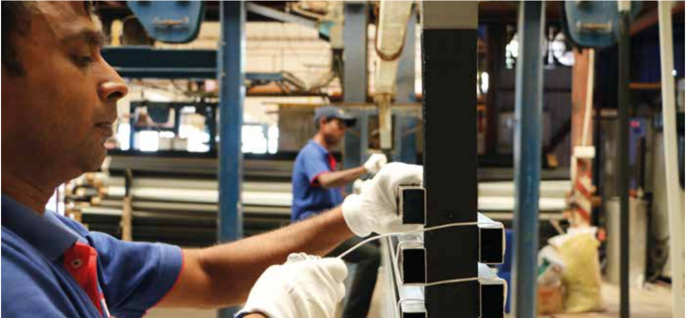
Preparation for aluminium anodizing process- Swisstek Aluminium Ltd Dompe
