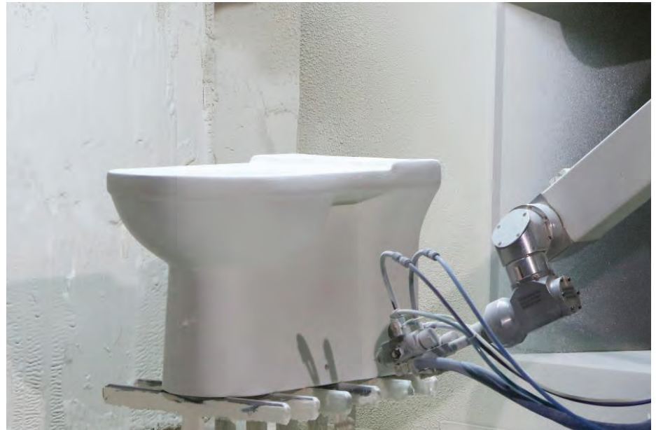
Robotised Glazing Machine – Rocell Bathware Godagama
